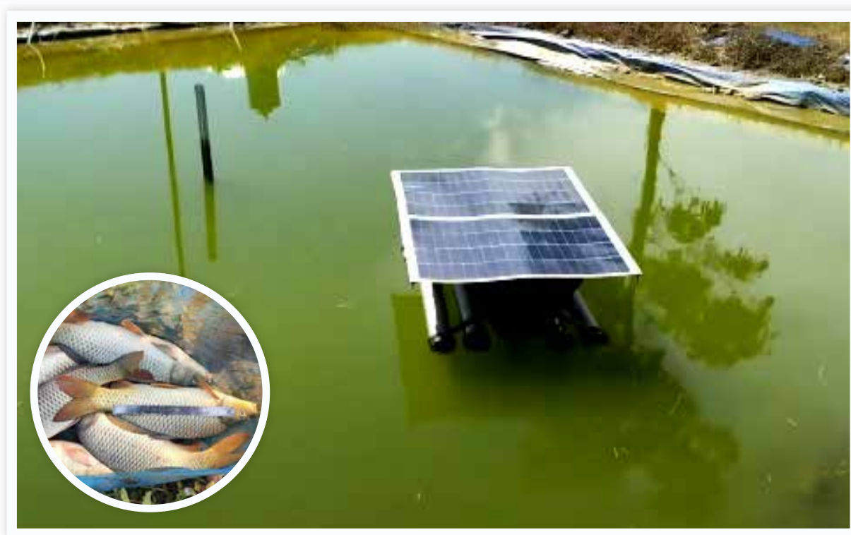
Solar powered feed dispenser-cum-aerator floating in pond
