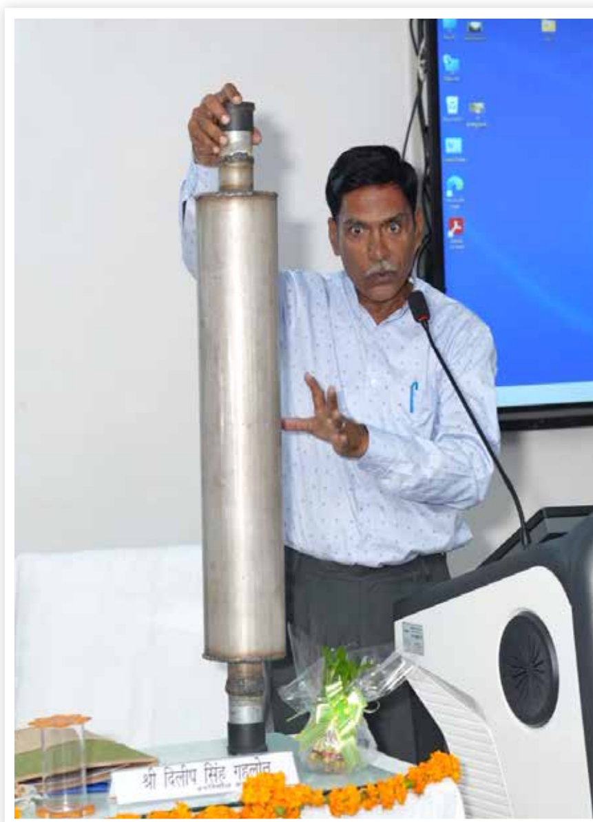
Magnetic water conditioner for treating saline water
