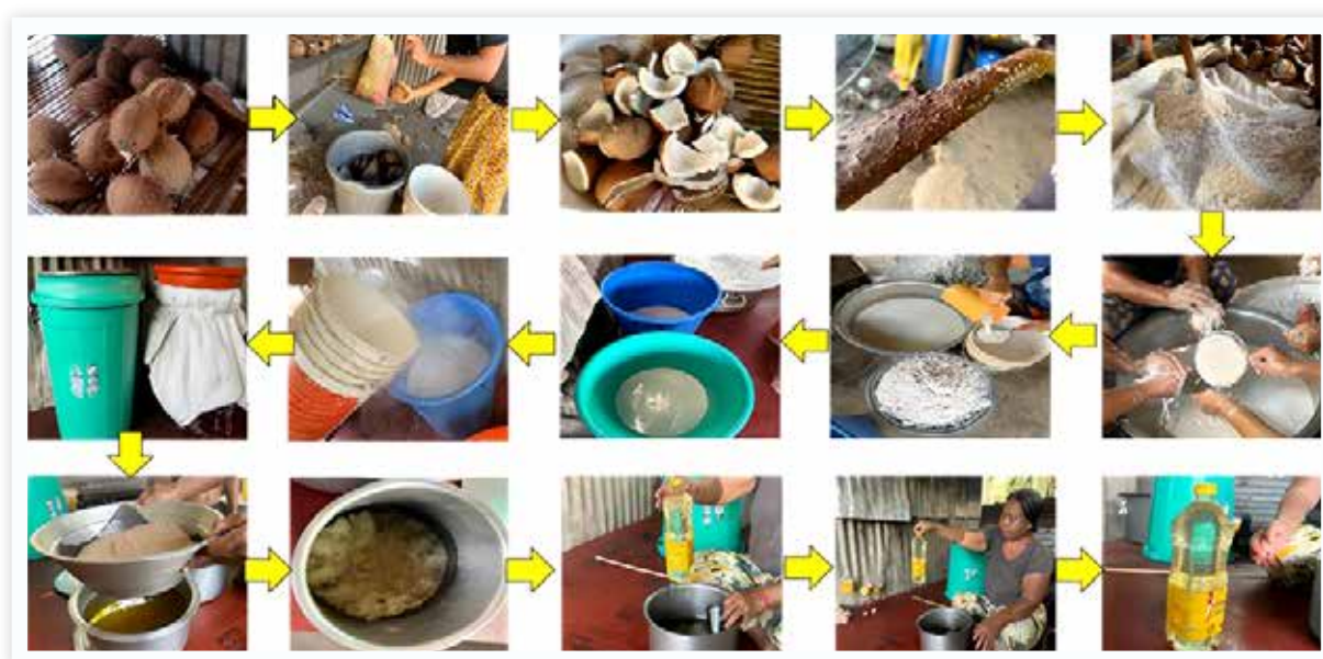
Process of tradition formation method of producing virgin coconut oil (VCO)
