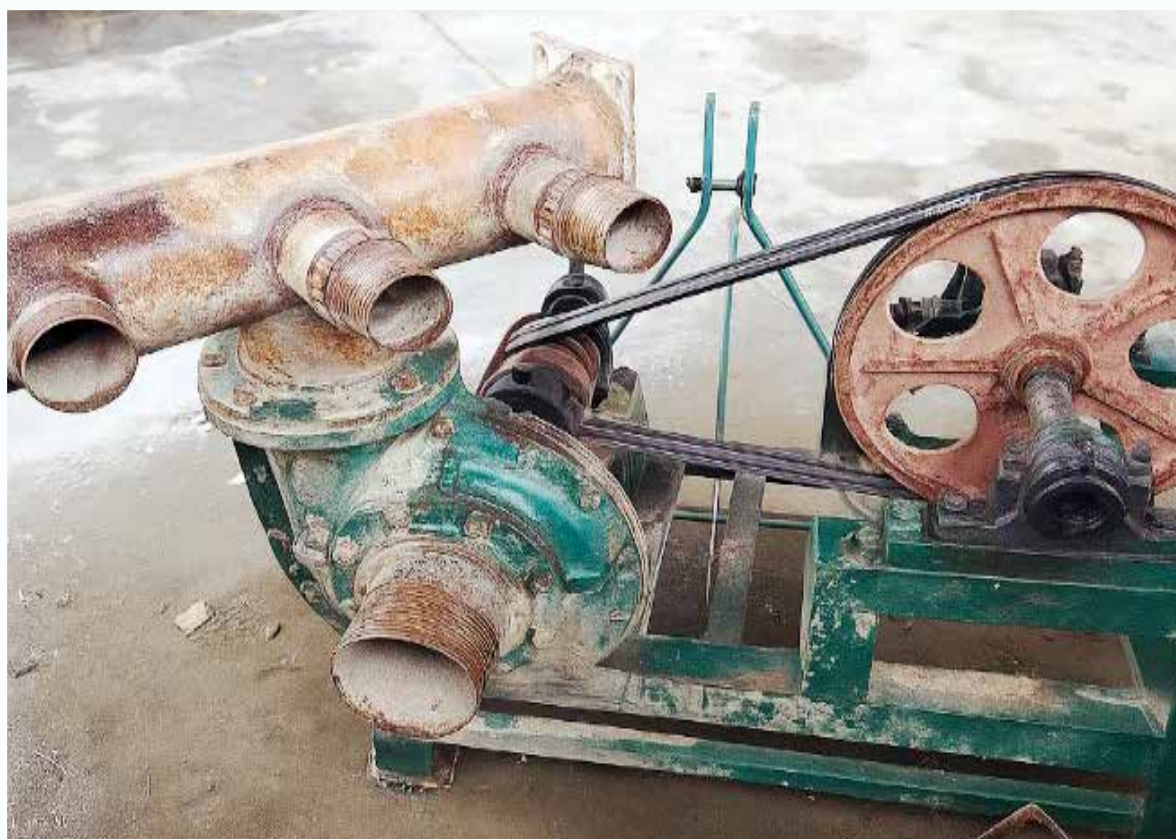
Modified water lifter
