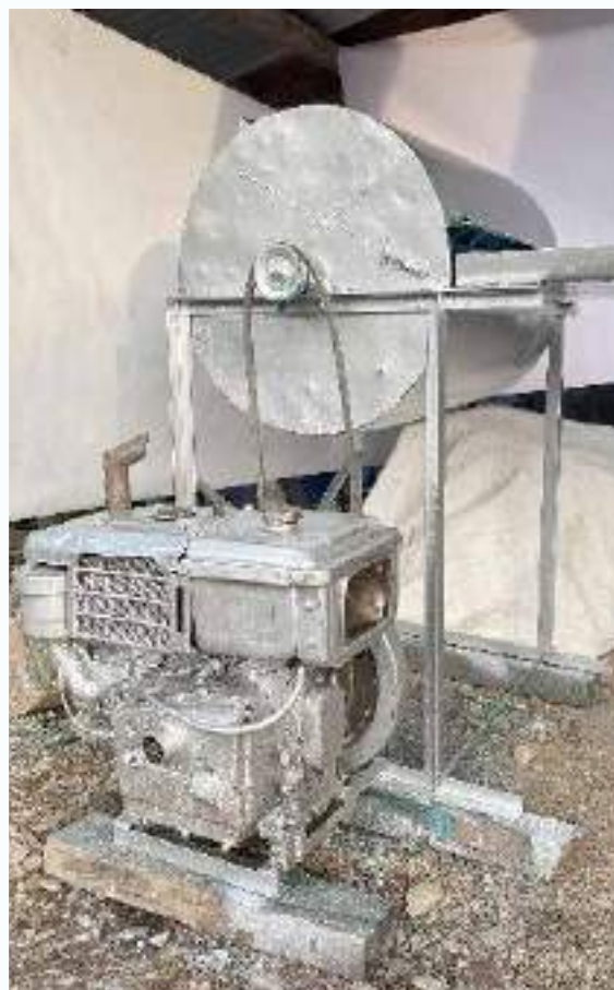
Diesel operated drum-type paddy thresher
