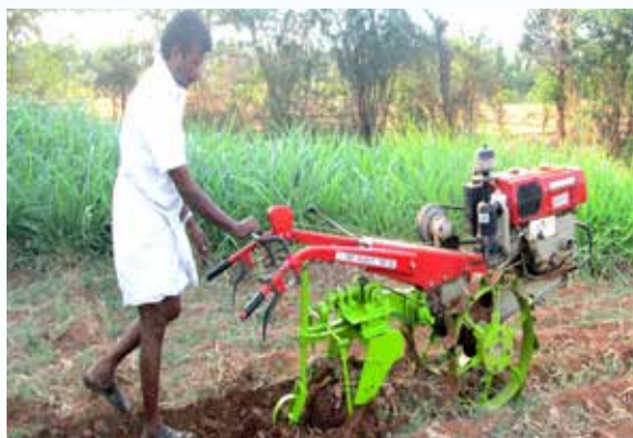
Power tiller-turmeric harvester in operation
