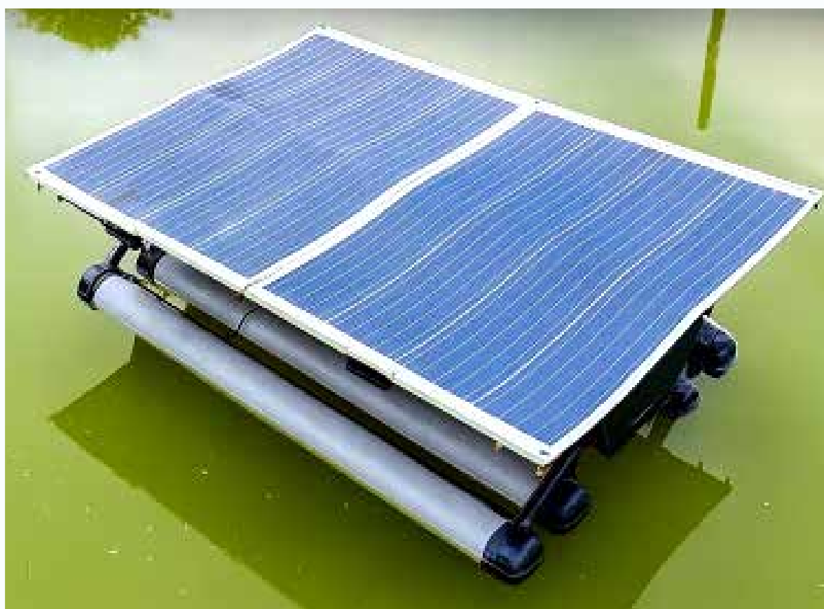
Solar powered float feeder-aerator
