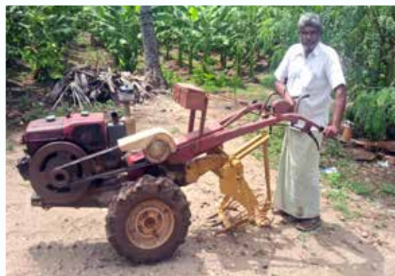
Power tiller-turmeric harvester in operation
