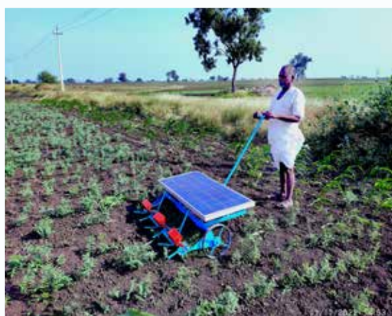
Solar powered plant nipping machine
