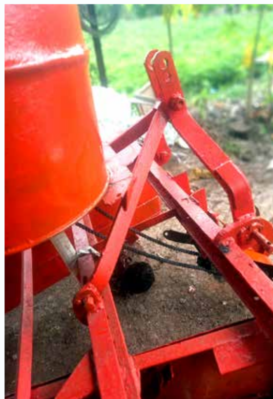
Ridge - bund maker with adjustable fertilizer application
