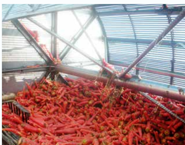
Inside view of a carrot washing machine
