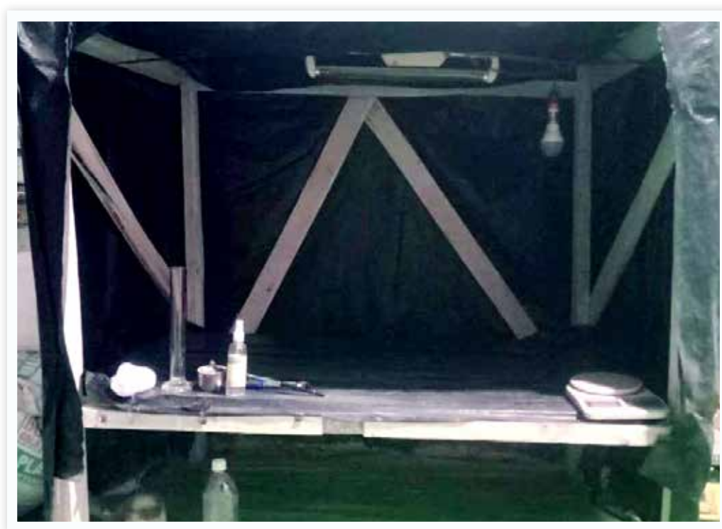
Low cost laminar flow cabinet for small scale Spawn production
