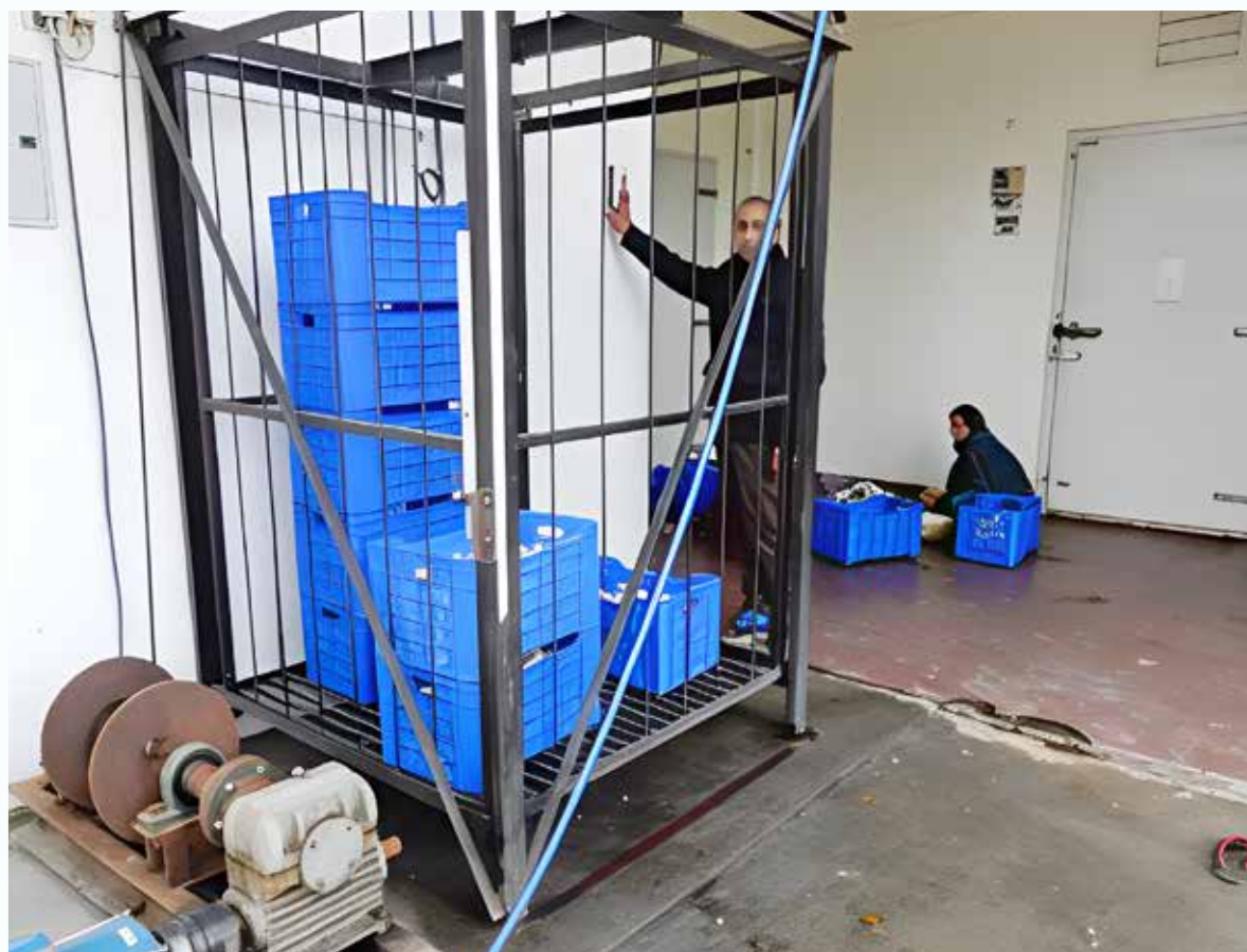
Close view of fabricated power lift
