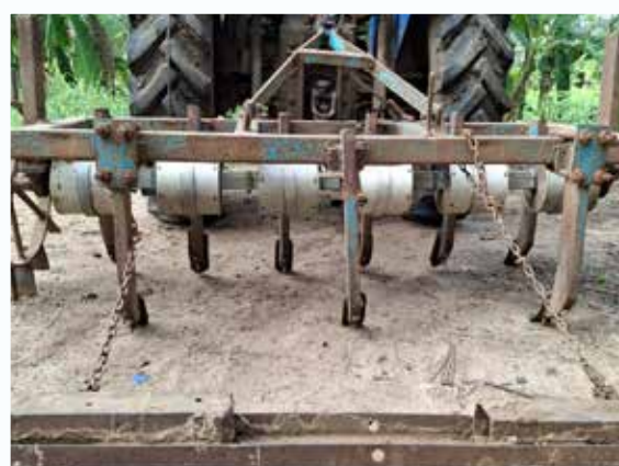
Close view of drum seeder cum cultivator cum planker
