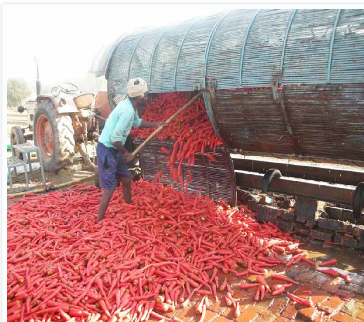
Unloading the carrot after washing in carrot washing machine
