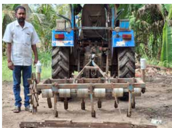
Close view of drum seeder cum cultivator cum planker
