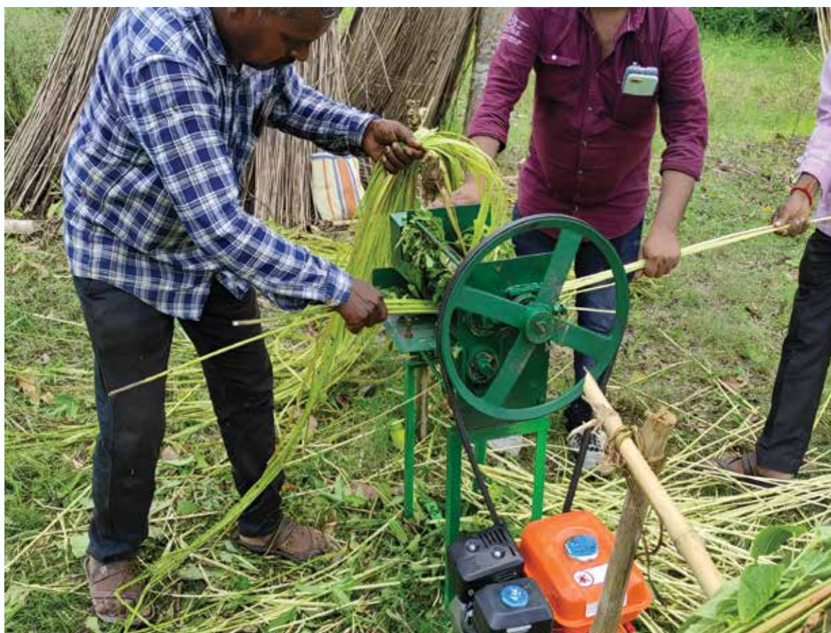
View of operation of Jute Ribbon Extractor machine
