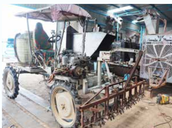
Custom built DSR machine fitted on jugad
