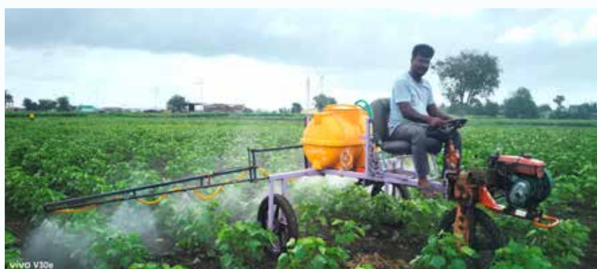
Mechanized weeder cum sprayer in action
