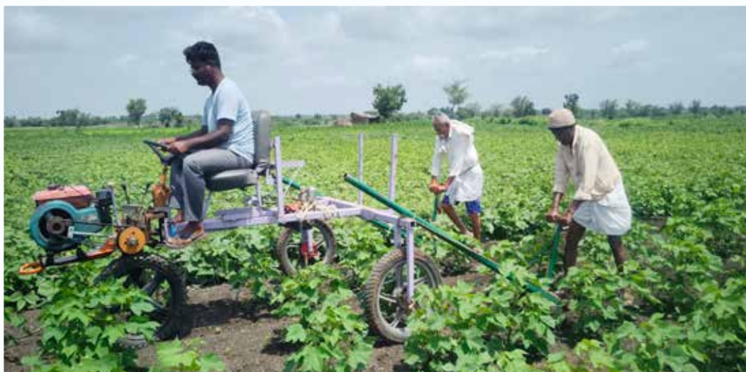
Innovator operating his weeder cum sprayer in the field
