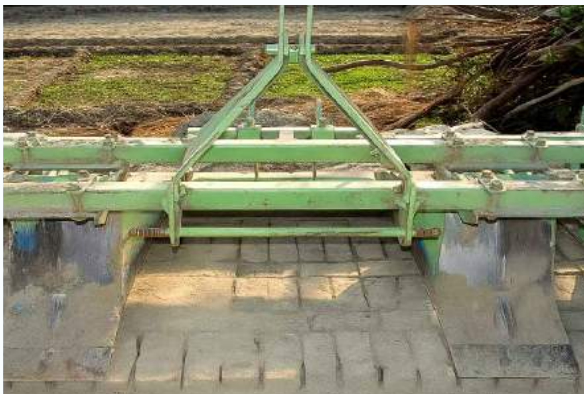
Modified sugarcane trench opener for mechanized irrigation
