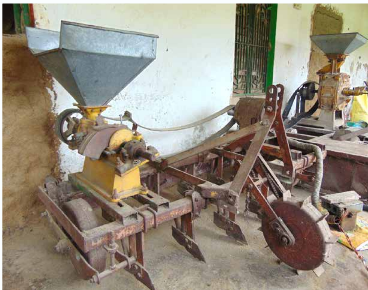
Rice huller fixed on zero-till machine
