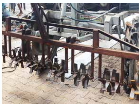
Custom built DSR machine fitted on jugad
