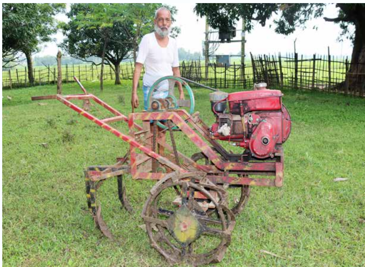
Low-cost power-tiller-cum-zero tillage machine
