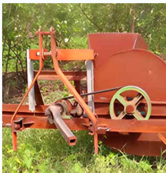
Different views of mechanized ber-shredder
