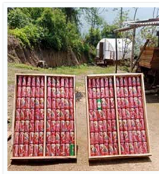
Recycled aluminium cans used in Solar dryer
