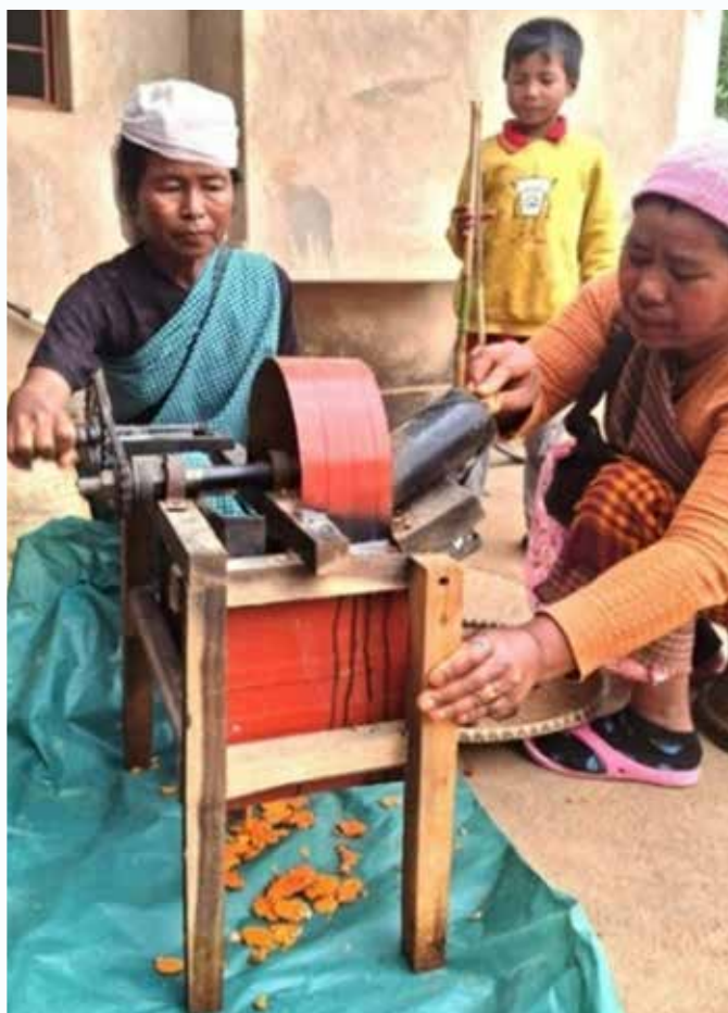
A view of ginger cum turmeric slicer under operation
