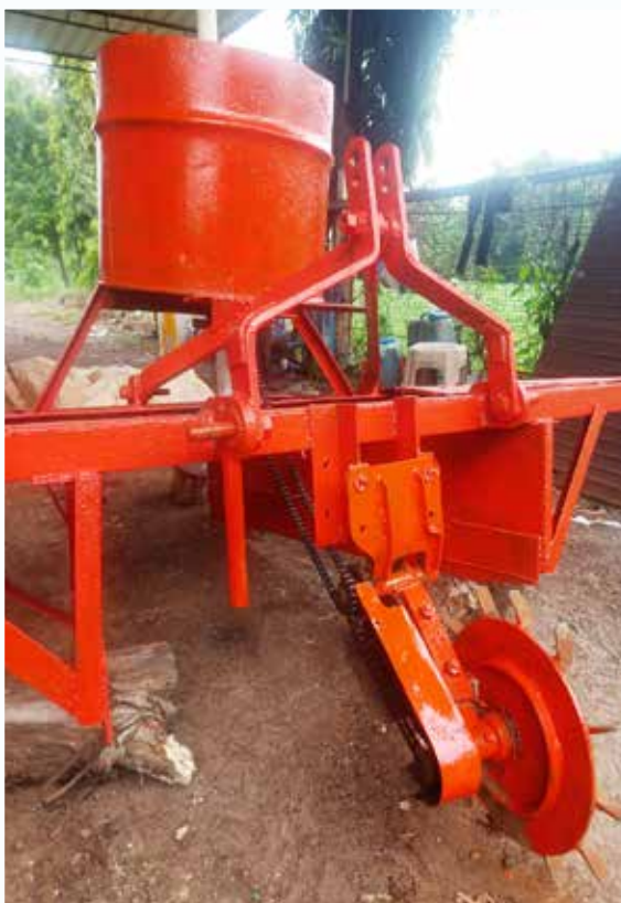
Ridge - bund maker with adjustable fertilizer application
